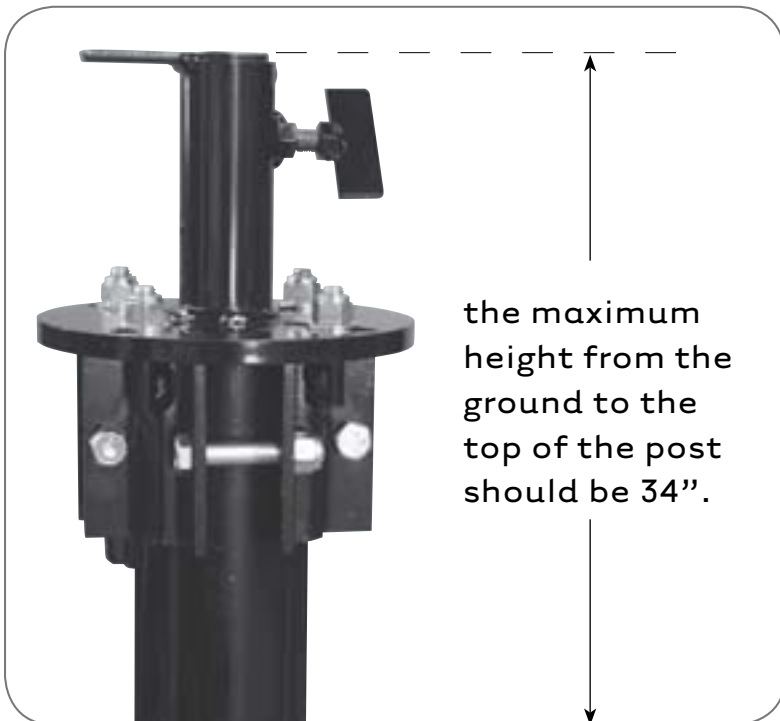
Figure 24 Slide unit over post and attach 4th bolt.
